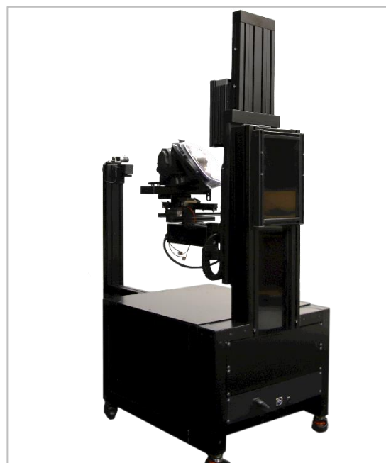
Fig. AUTO 50.A goniometer with BTC 2000 accessories. Max DUT size 0.6 m (length), 0.25 m (height), 5kg.
